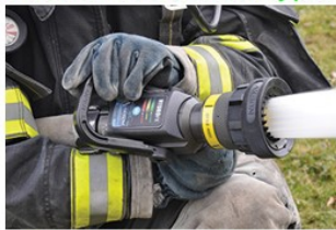
Combination nozzle on tight straight stream setting
